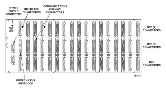
Figure 6-1. RDC-01/02 PatchSwitch Chassis Rear View
